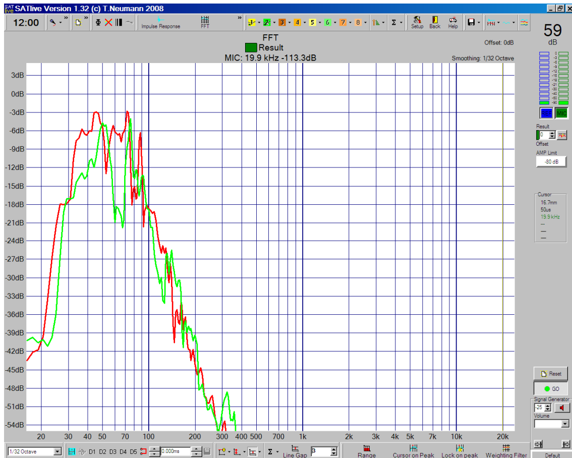
Fig. 29. This image compares the pressure curve of the forward facing subwoofers at the measurement microphone (red trace) to the cardioid configuration (green). In this case, there is a band where a difference of up to 6dB can be seen and another band with differences up to 9 dB .
