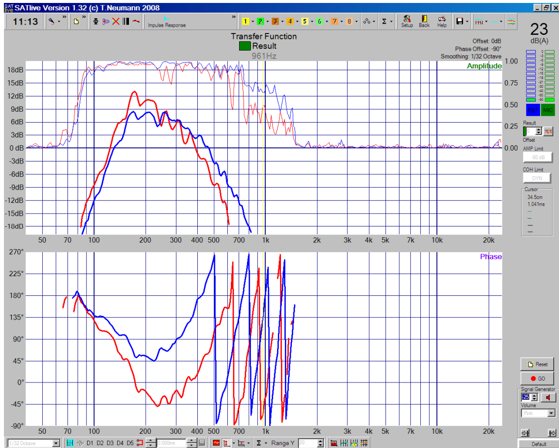
Fig. 16. Comparison of forward facing (red) and backward facing (blue) subwoofers. As expected, differences in phase and level can be noted.
